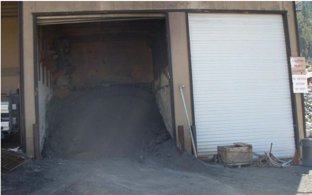
*Abrasives and deicers should be stored on a paved surface and covered on the top and three sides to protect the material from precipitation and wind.*
