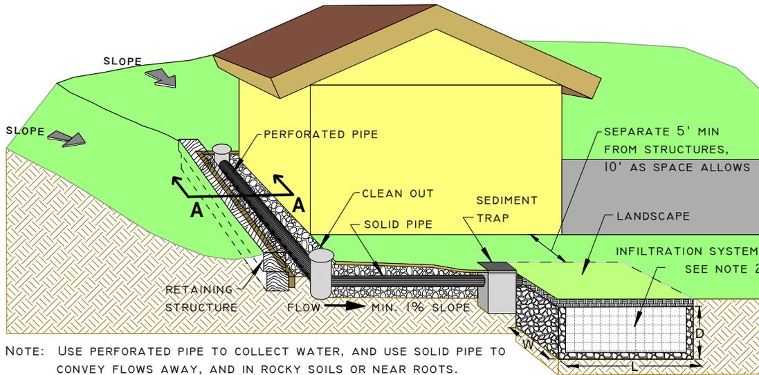
NOTE: USE PERFORATED PIPE TO COLLECT WATER, AND USE SOLID PIPE TO CONVEY FLOWS AWAY, AND IN ROCKY SOILS OR NEAR ROOTS.
