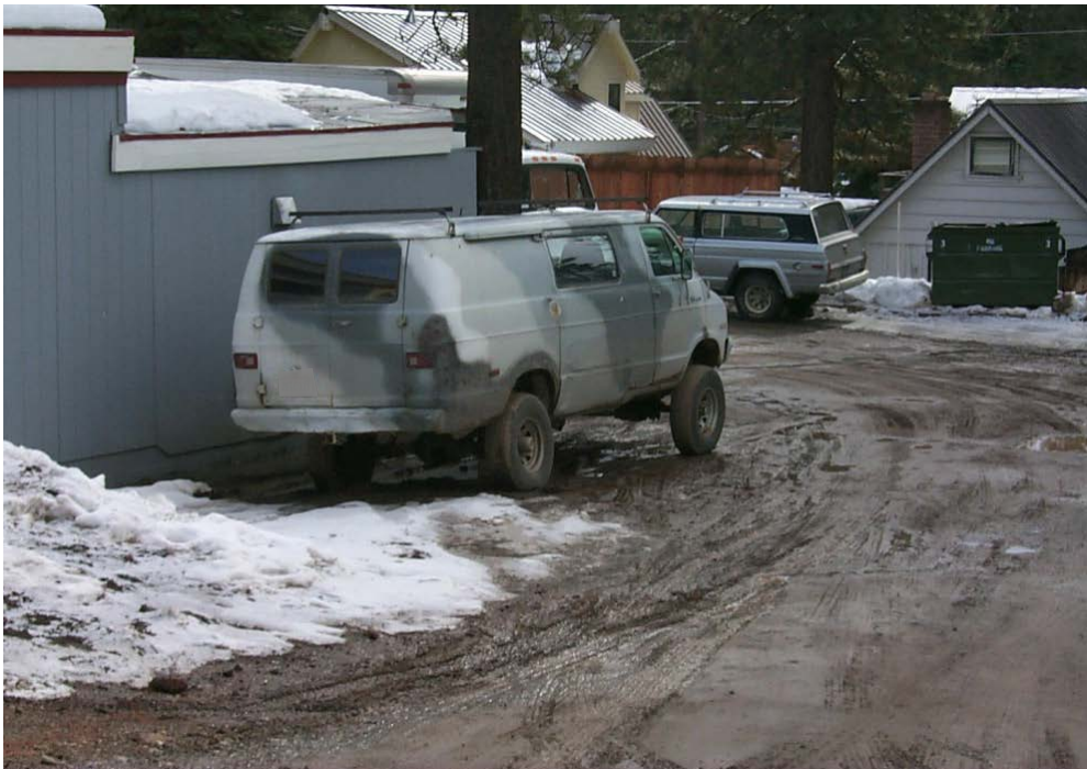
Parking off of paved surfaces compacts the soil, preventing stormwater from naturally infiltrating and causes erosion and sediment laden stormwater runoff.
