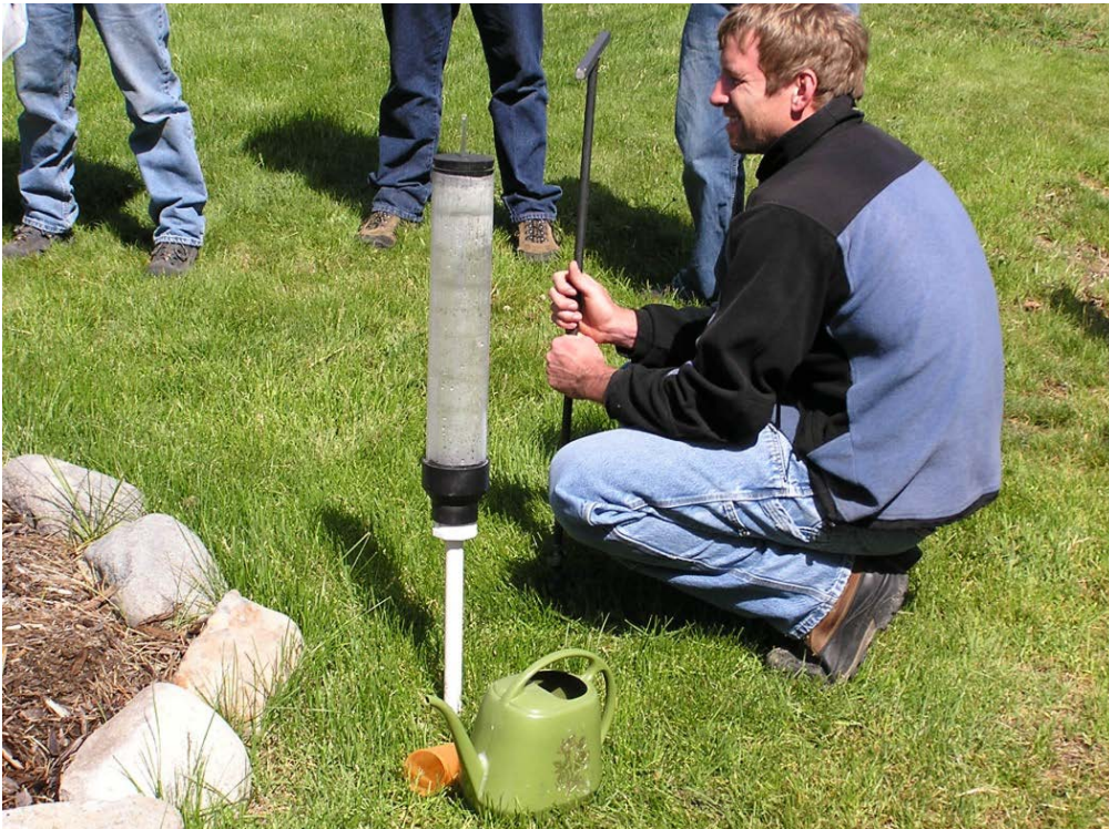
A Constant Head Permeameter (CHP) test being conducting on a residential site to determine the on-site Ksat of the soil.
